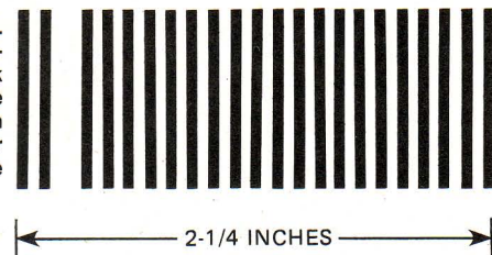
FIG. 14—THE FOIL PATTERN for the double-sided piggyback extender board. Note that only one pattern is shown. The other side is, of course, the same.
